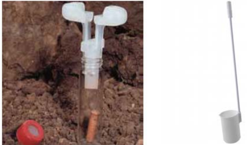
Figure 4. Environmental Collectors (left to right): QEC Terra Core Sampler, New Star Environmental Dipper
