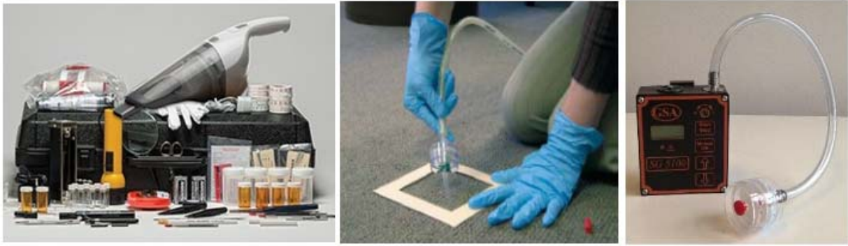
Figure 16. Vacuum/Aerosol Sample Collection Kits (left to right): Sirchie Evidence Collection ID, Sealing Kit, SKC Carpet Sampling Cassette Kit, and HotZone Aerosol Module
