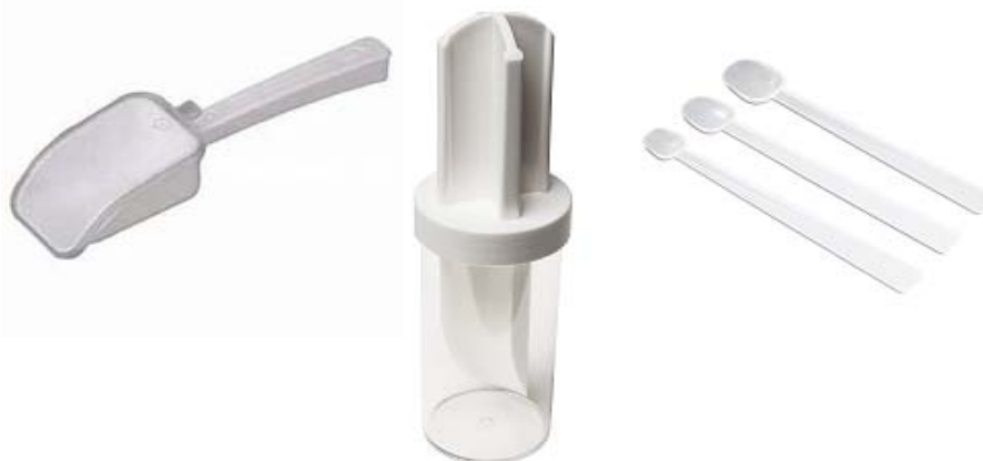
Figure 9. Scoops and Spoons (left to right): Burkle Sampling Scoop, Bel-Art Samplit Scoop and Container System, Bel-Art Sampling Spoons
