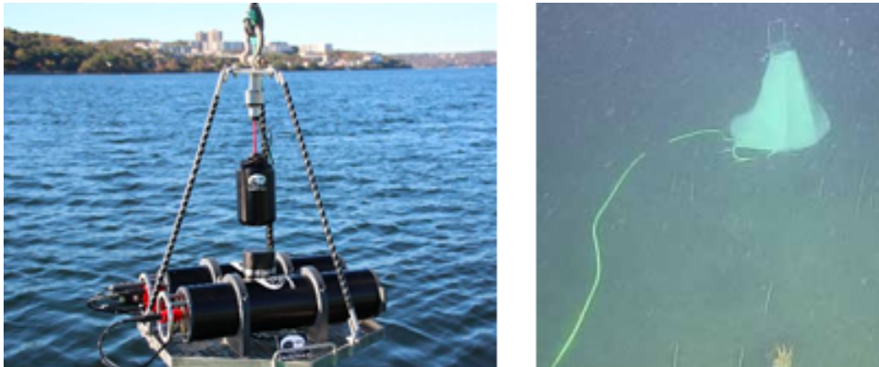
Figure 2.1. Left: MARS hydrophone preparing to submerge. Right: MARS hydrophone fully underwater. Source: Dawe and Ryan (2006).
