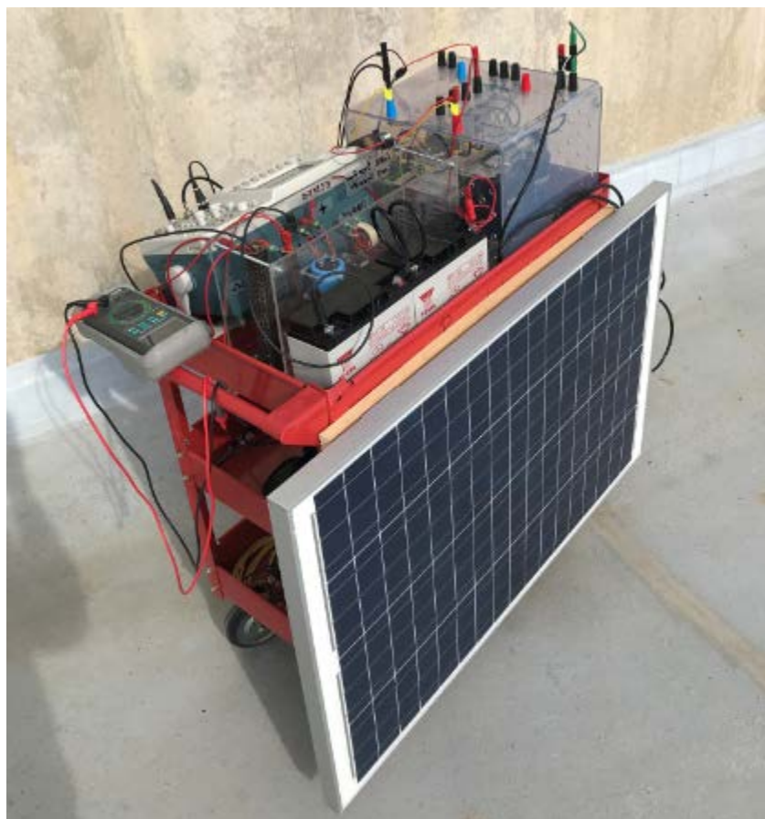
Figure 28. PV power system experimental configuration
