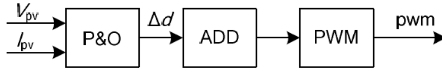
Figure 14. Control schematic of duty cycle P&O for MPPT. Source: [22].
