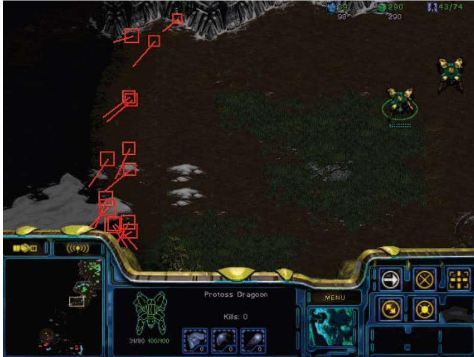
The EISBot playing as the green Protoss units. The red squares represent predictions of opponent positions and velocity for units that have moved out of visual range.
