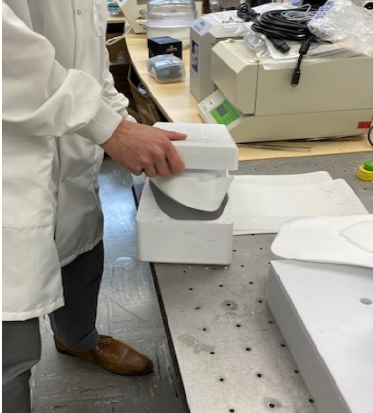
Figure 8. The author is shown removing composite pieces from the mold. Source: [9].
