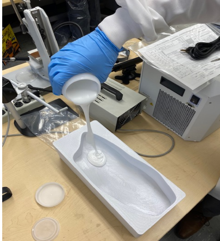
Figure 7. Demers pouring liquid composite into the bottom piece of a mold. Source: [9].
