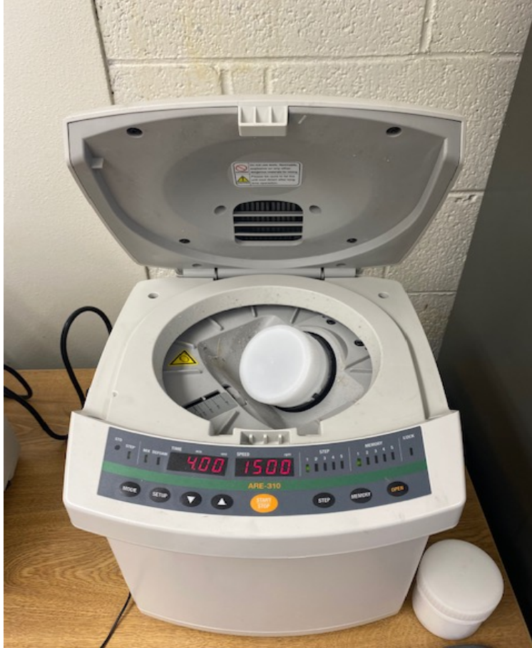
Figure 5. THINKY rotary mixer with jar inserted and set spin duration to be four minutes and spin frequency to 1500 rpm. Source: [9].
