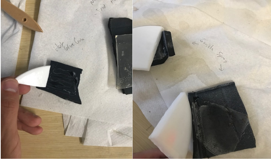
Figure 10. Glue adhesives that were used to adhere neoprene and our composite material.
