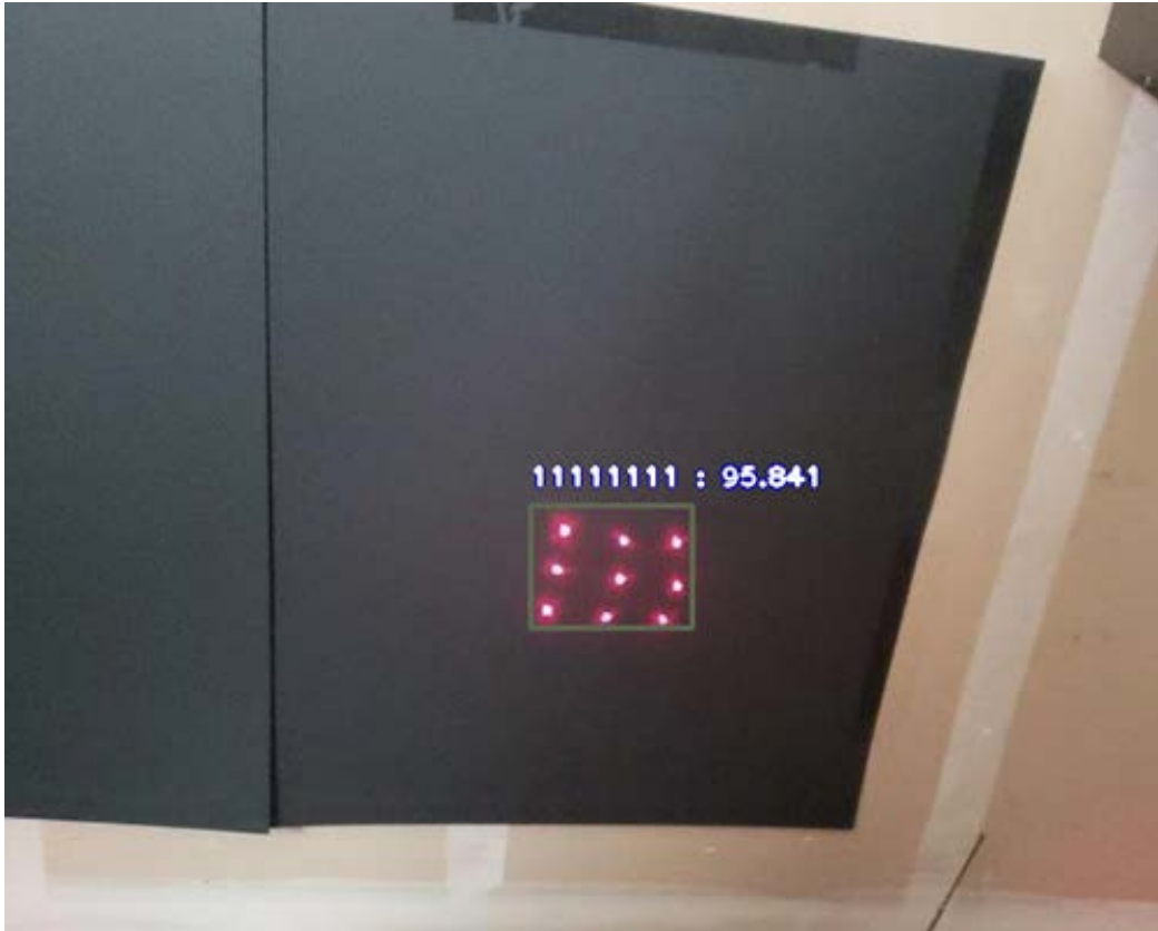
Figure 19. Image of a byte pattern reflected from FSO transmission with a 96% probability.
