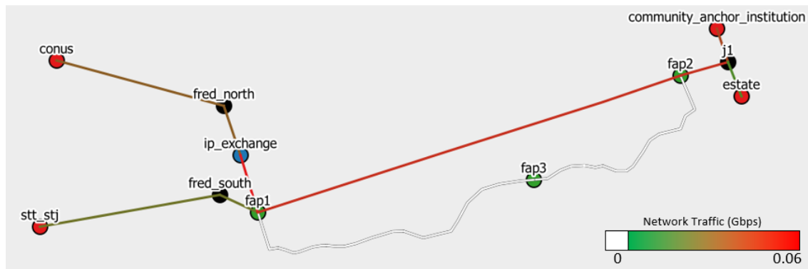
Figure 3.13. Layer 1 Traffic Assignment in Simple Model, All Edges Available. Aggregate traffic over layer 1 edges with all layer 1 edges available. White lines indicate no traffic flow. Traffic flow over edges increases from green to red as the amount of traffic flow over the layer 1 edge increases.
