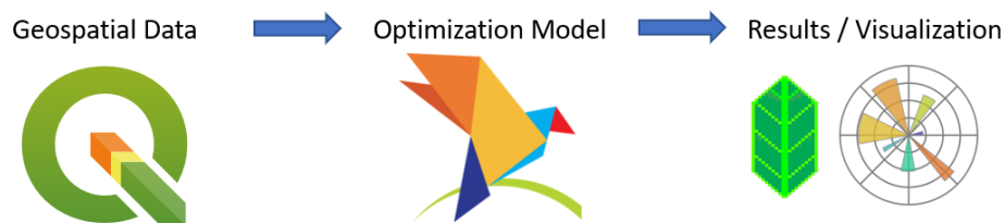
Figure 3.1. Diagram of the project's workflow. We develop and curate a geospatial dataset using QGIS. We then use Pyomo to solve the optimization model detailed in Section 3.3. Finally, we plot the resultant maps and graphs using Folium and matplotlib, respectively.
