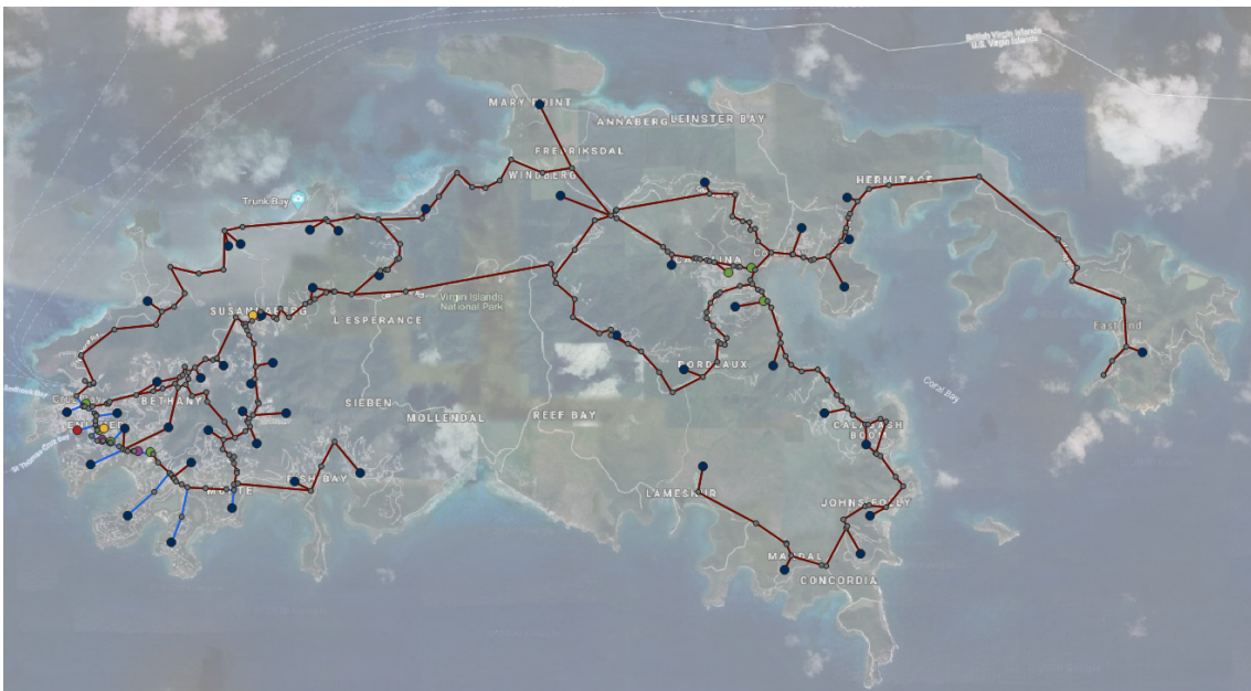
Figure 4.1. STJ model road network. “Urban” roads are in blue. “Winding” roads are in burgundy. Created using QGIS Development Team (2020) on 18 September 2020.
