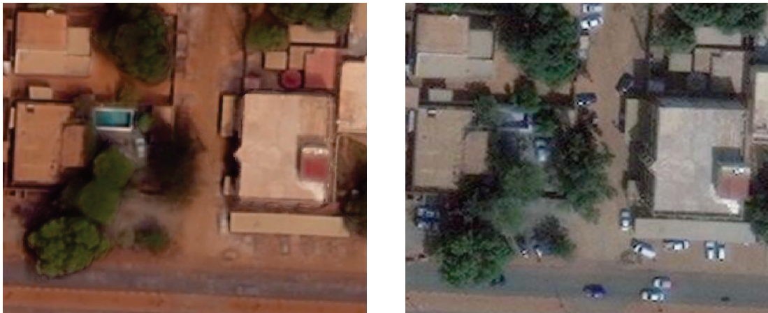
Figure 5. A 1:500 scale comparison of the imagery used in Niamey for digitizing (left) and ArcMap Basemap (Esri n.d.) (right). While the images are not from the same date the difference between the images does reveal the distortion present in the digitizing image. Distortion is most evident along roadways where cars are barely visible as well as in the blurring around trees.
