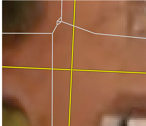
Figure 6. A 1:100 scale example of Tier 2 road layer generated excessive line segments. The white lines are Tier 2 generated road segments while yellow lines are manually digitized roads. Tier 2 AFE generated a series of small segments in a triangular pattern in place of a standard cross intersection.
