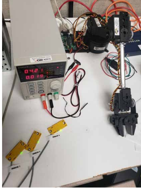
Figure 5. DIOL proximity sensors and control arm (in the secured position)
