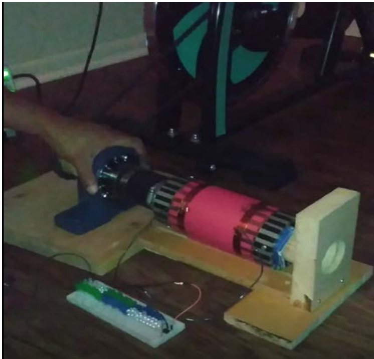
Figure 56. 120 LEDs connected to TENG with Stationary Bike
