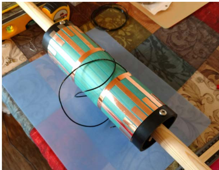
Figure 14. TENG Model (1.27cm Copper Taping)
