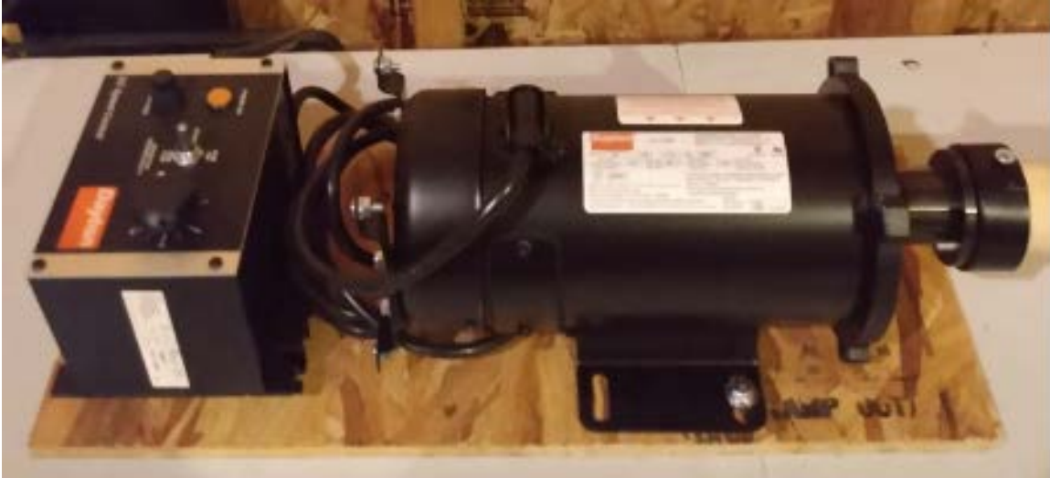
Figure 10. Dayton PMDC Motor with Controller (Model: 2Z846)
