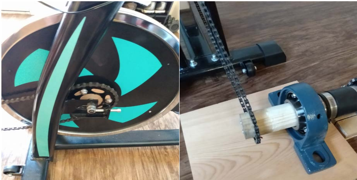
Figure 53. Stationary Bike with Mounted Gears and Chain
