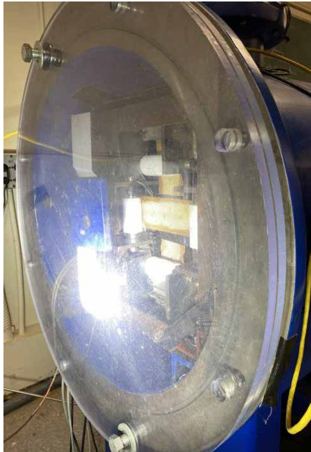
Figure 24. Clear polycarbonate plates attached to catch tank.
