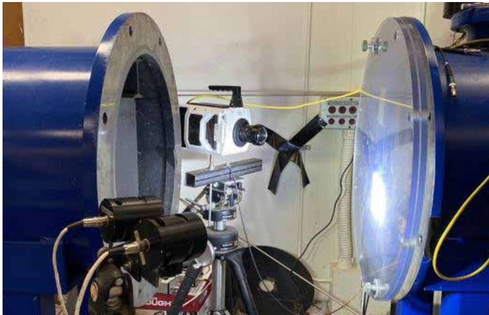
Figure 23. Camera and lighting setup for experiment image capture.
