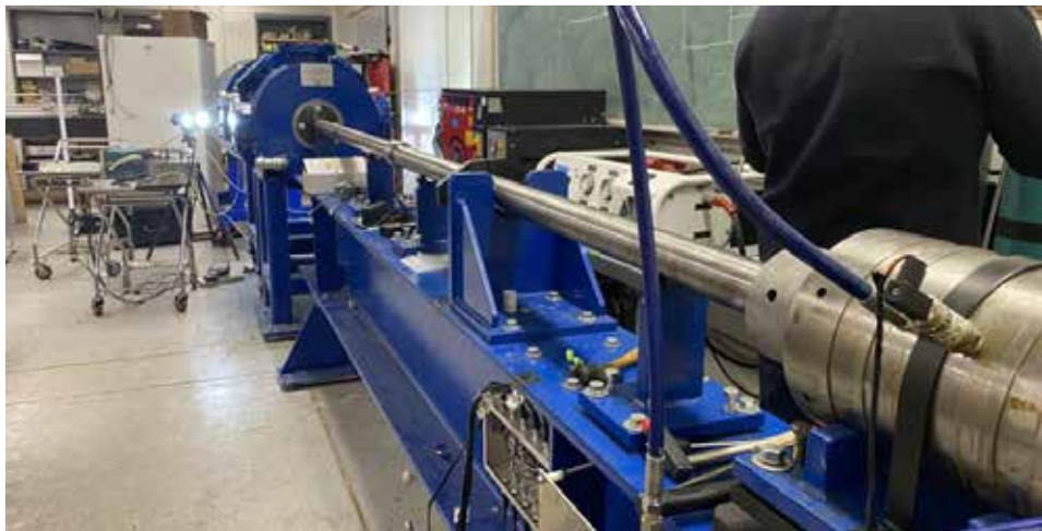
Figure 15. Breech, barrel, and catch tank of the light gas gun.
