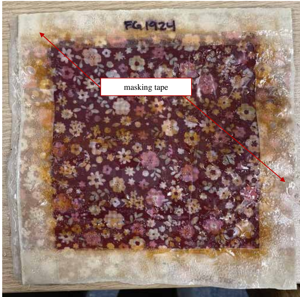
Figure 9. Placement of tape around edges of coating sample.
