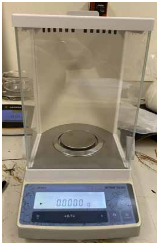
Figure 29. Mettler Toledo AB104-S analytical balance, used for measuring mass of PBO wefts.
