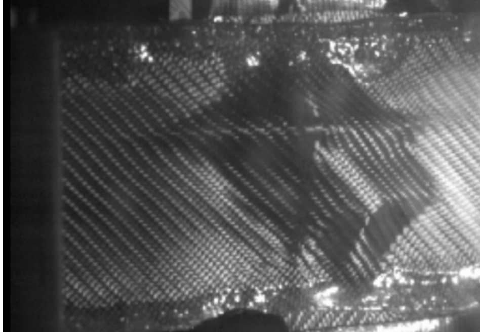
Figure 37. Moment of peak deflection for uncoated unexposed PBO.
