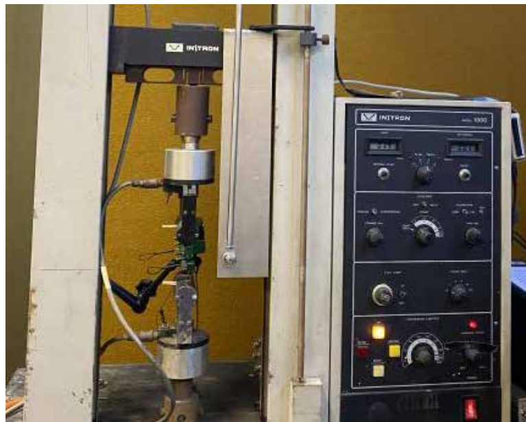
Figure 14. Instron tensile testing machine with attached load cell for elongation measurements.
