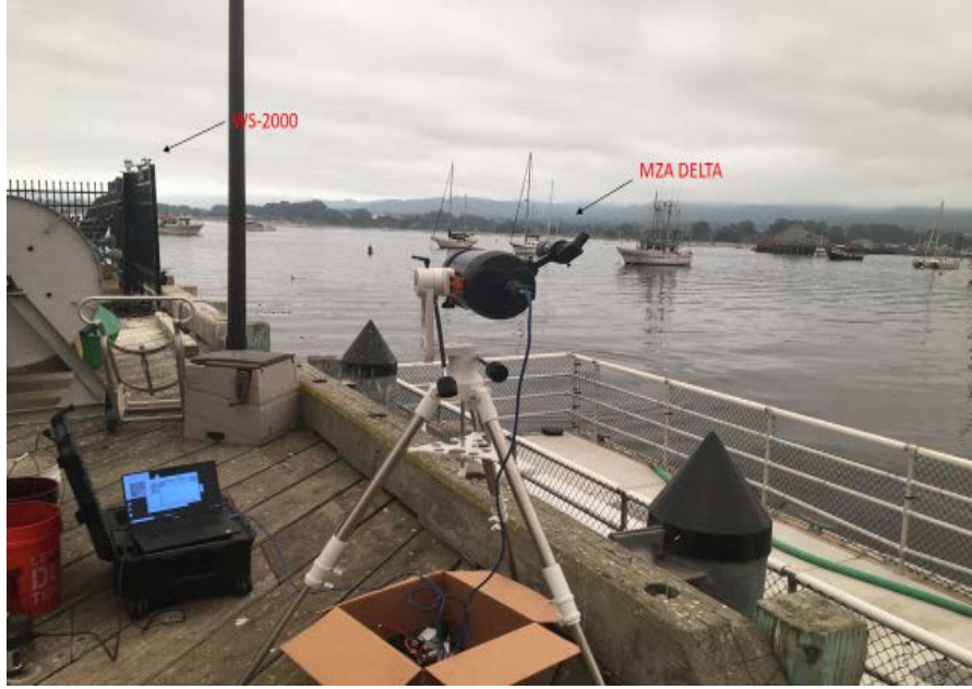
Figure 20. The DELTA sensor as well as the WS-2000 weather station set up at the CG Pier
