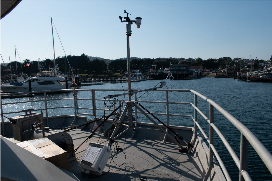
Figure 24. The CSAT3 sonic anemometer, with the WS-2000 mounted on top of it, on-board NOAA ( Fulmar ) ship
