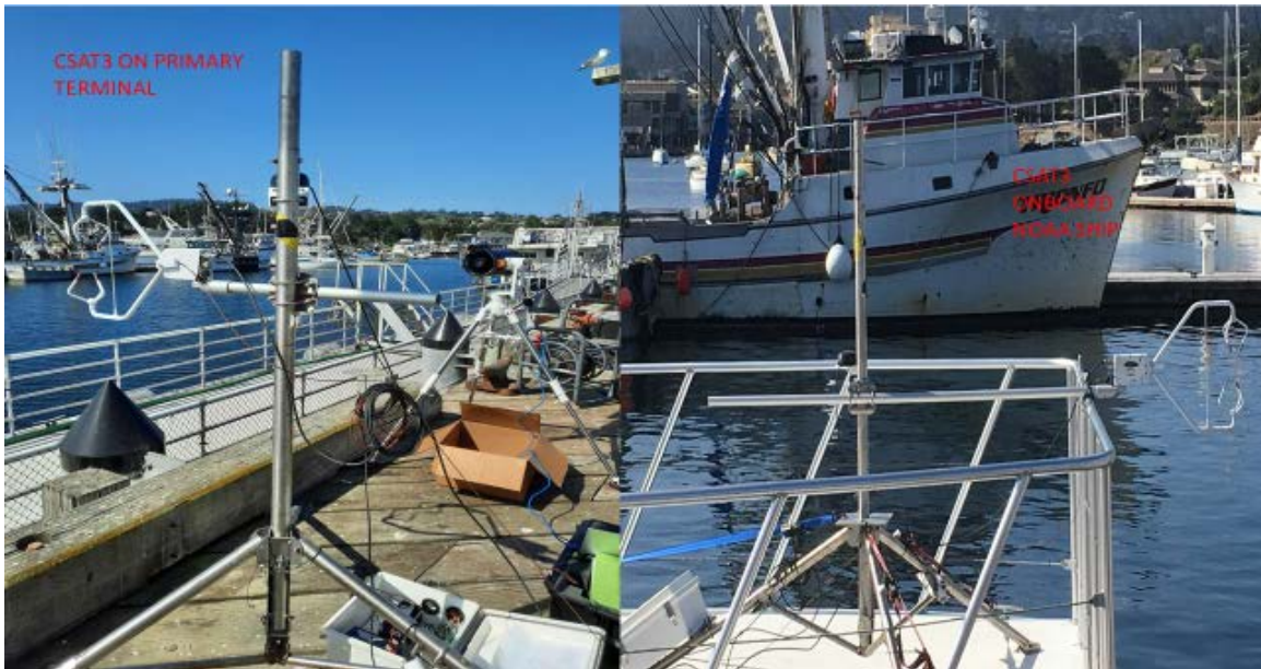
Figure 22. The CSAT3 sonic anemometers at the CG Pier (left) and on-board NOAA ship (R4017) (right).
