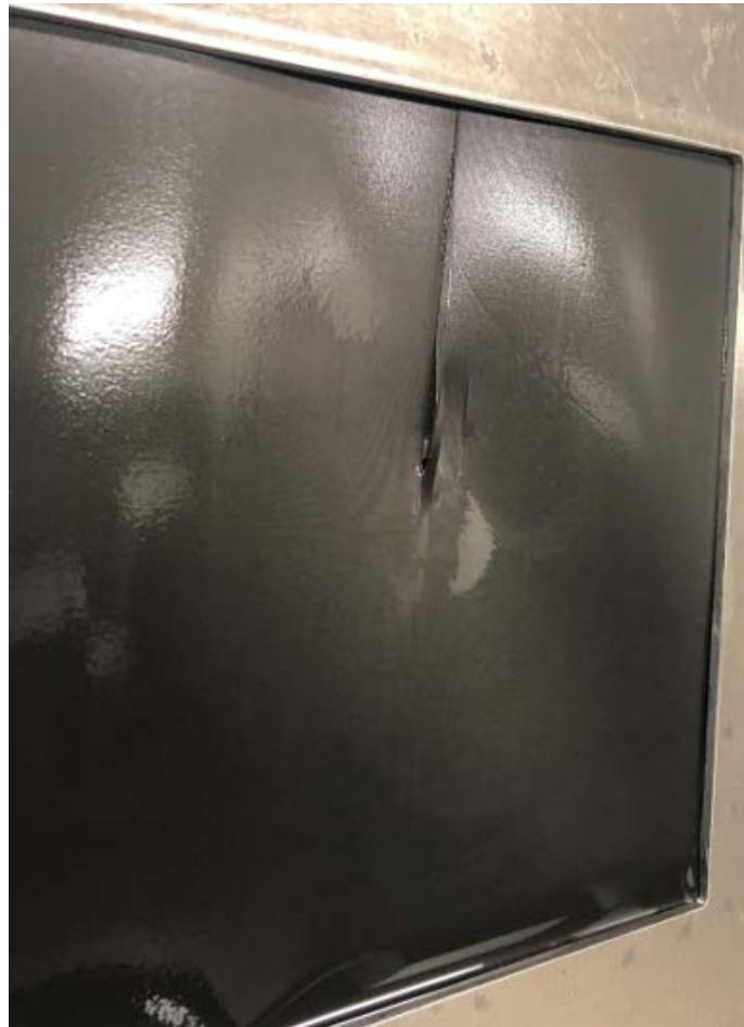
Figure 94. Sample 4 set-up 3 after 3 rd blast
