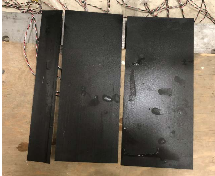
Figure 73. Sample 2 failure after 2 nd blast
