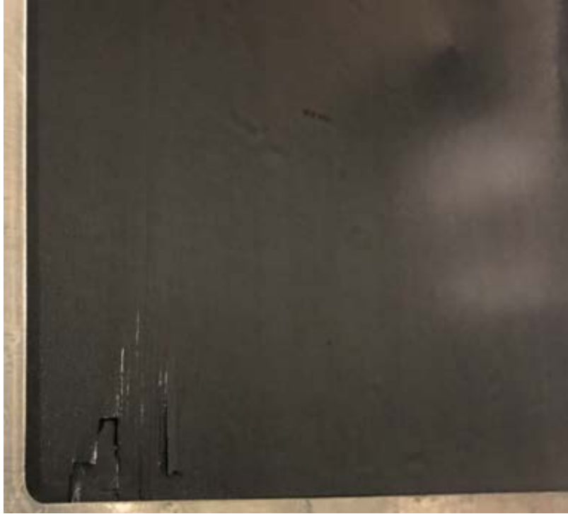
Figure 91. Sample 4 failure after 2 nd blast
