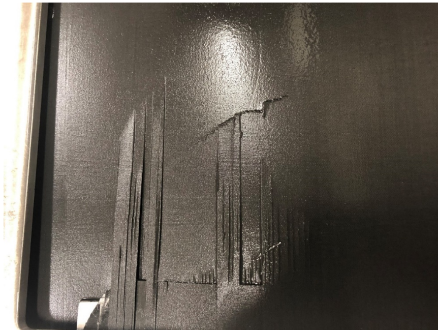
Figure 93. Sample 4 failure after 3 rd blast
