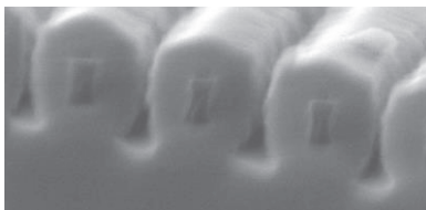
Fig. 1b. Scanning electron microscope (SEM) picture of a wire structures ( \sim 75\text{nm} ) after thermal oxidation.
