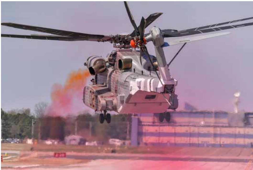
Figure 17. Colored Oil Smoke Test Identifies Cause of Engine Gas Re-ingestion Issue. Source: Eckstein (2019b).
