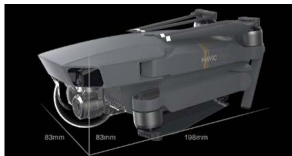
Figure 6. Folded DJI Mavic Pro with Dimensions. 50
