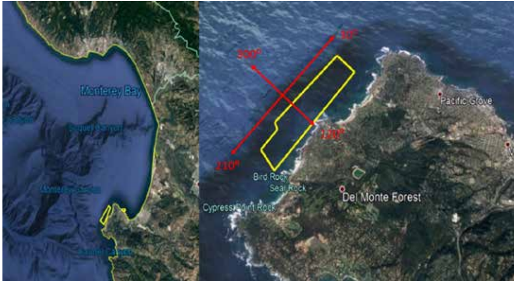
Data were collected within the yellow box in a lawnmower type pattern near Asilomar Beach Monterey, CA in 2019. The beach is angled approximately 30^\circ from north. Alongshore headings are 30^\circ and 120^\circ and cross-shore headings are 120^\circ and 300^\circ .
