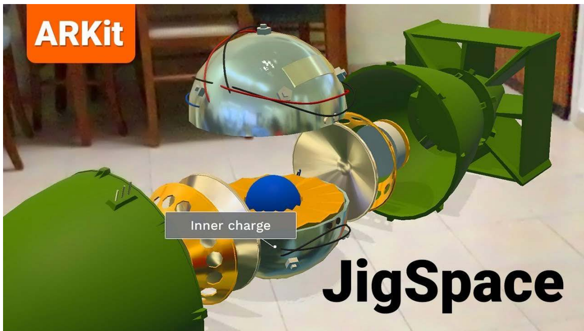
Figure 11. Exploded view of mechanical device in AR. Source: AR Critic (2017).
