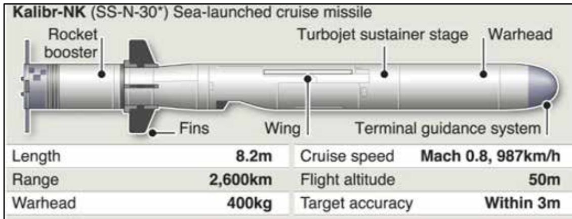
Figure 2. Russia's Kalibr-NK (SS-N-30A SAGARIS also known as 3M-14 Kalibr) Sea-Launched Cruise Missile Specifications 173
