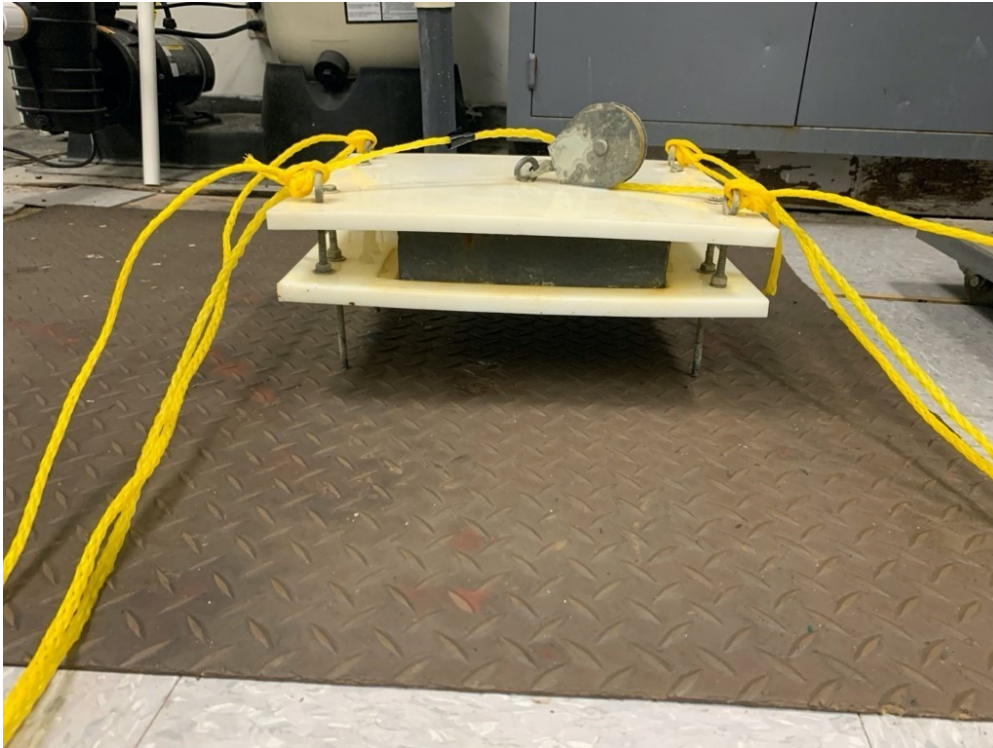
Lead bricks are sandwiched between plastic plates. A cord passing through the pulley is used to alter balloon depth. Cords around exterior are for adjusting the placement of anchor system. 6-inch bolts are used as stilts.
