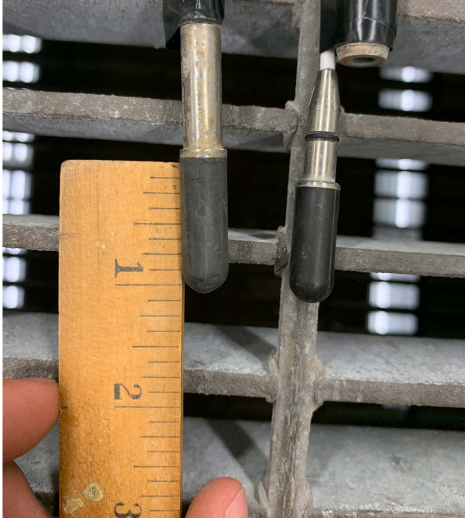
Left: Unknown cylindrical hydrophone used as an acoustic projector Right: B&K 8103 hydrophone used as an acoustic receiver
