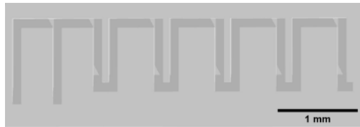
Figure 11. SOLIDWORKS model of a Wi-Fi antenna subtracted from a block
