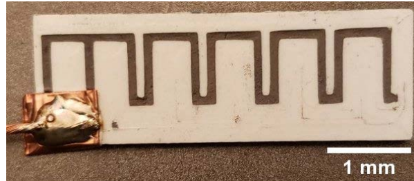
Figure 24. Ti-64 composite Linksys antenna
