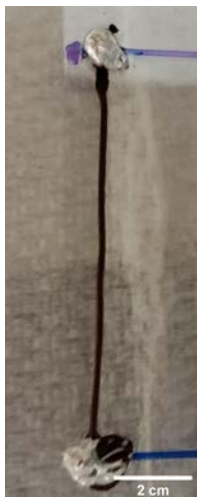
Figure 5. Copper (Cu-110) epoxy composites on glass slide with solder ends
