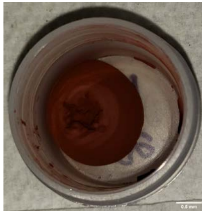
Figure 2. Copper (Cu-110) mixed with two part epoxy at 93% by weight
