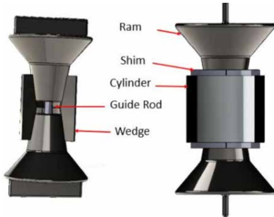
Figure 10. Wedge and Ram Testing Device. Source: [6].
