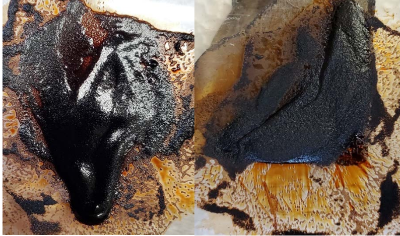
Left: fluid-like, no magnetic field; right: solid-like, magnetic field present
