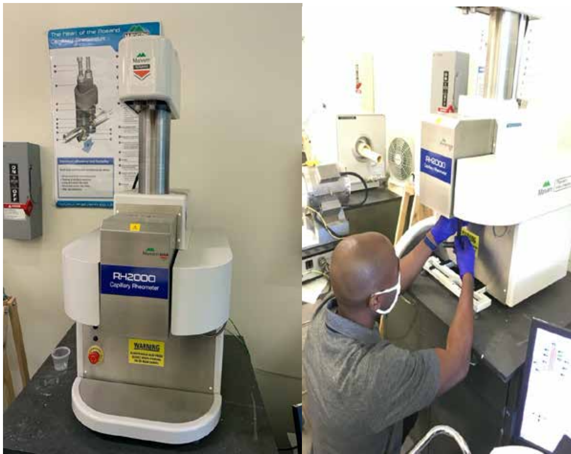
Figure 23. (Left) Capillary rheometer (Rosand RH2000) (right) Installation of die.
