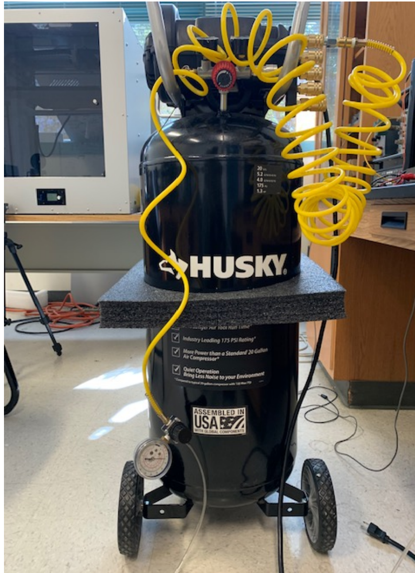
Figure 28. 75-liter air compressor assisted with an air regulator used
