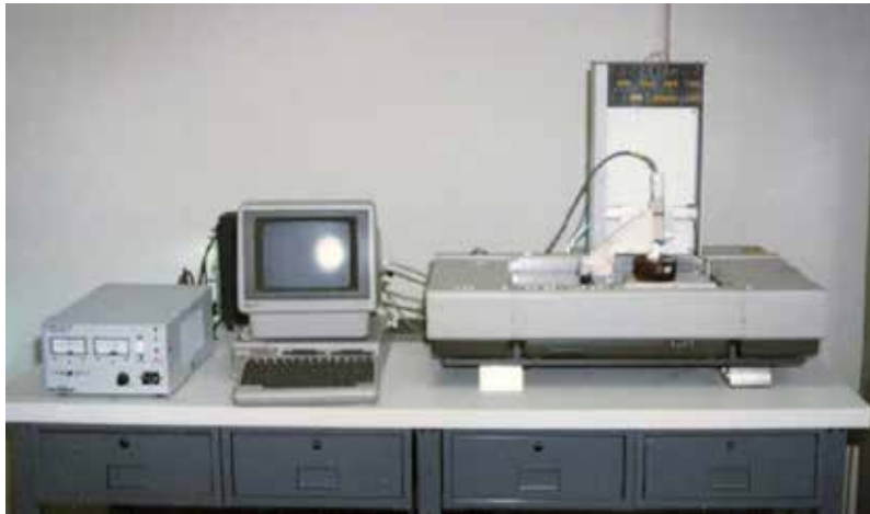
Figure 3. The first 3D printer, invented by Charles Hull. Source: [13].
