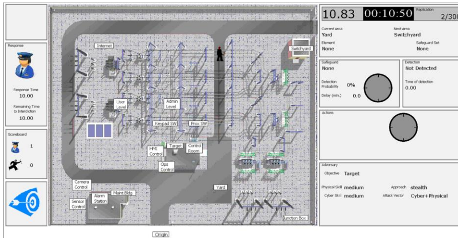
PACRAT's User Interface (the “dashboard”) and the output display (with color coded, statistical pathway analysis)
