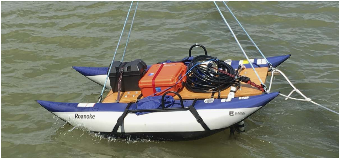
Figure 12. The Banshee deployed from the ship's crane alongside the R/V Virginia on 24 April. The 12 vdc marine battery is in the black box on the left, the BioSonics electronics is housed in the orange watertight case and the excess cable is secured on the right.
