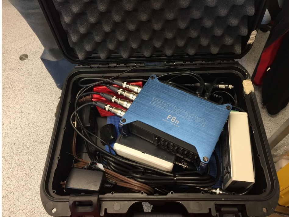
Figure 9. The electronics inside the watertight case shown on the mini-cat in Fig. 8. The case contained the Zoom F8n 8-channel recorder (blue), the 8-channel pre-amp (gray/white), the GPS time-code generator (cream) and the 12v inverter (red).
