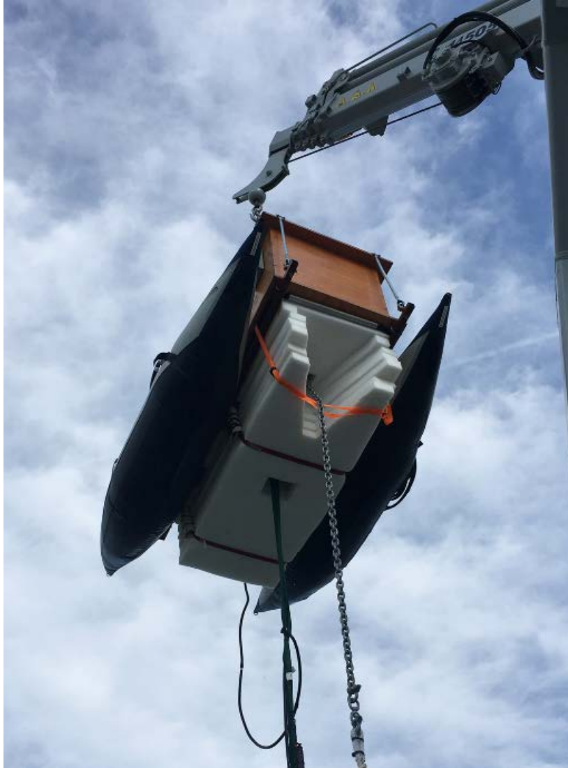
Figure 10. The underside of the "coffin" (hanging from the ship's crane) showing the additional floatation, the anchor chain/line and the line from which the acoustic source was suspended.
