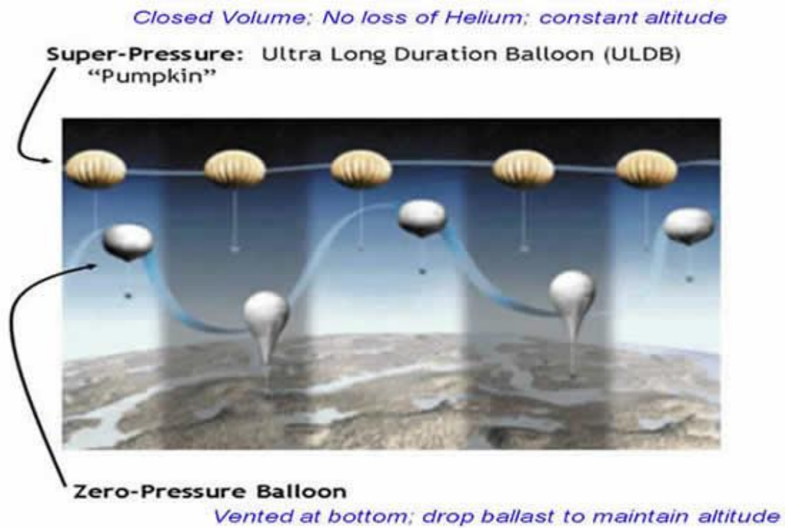
Fig. II-6. Zero-pressure and super-pressure balloons comparison [41].
