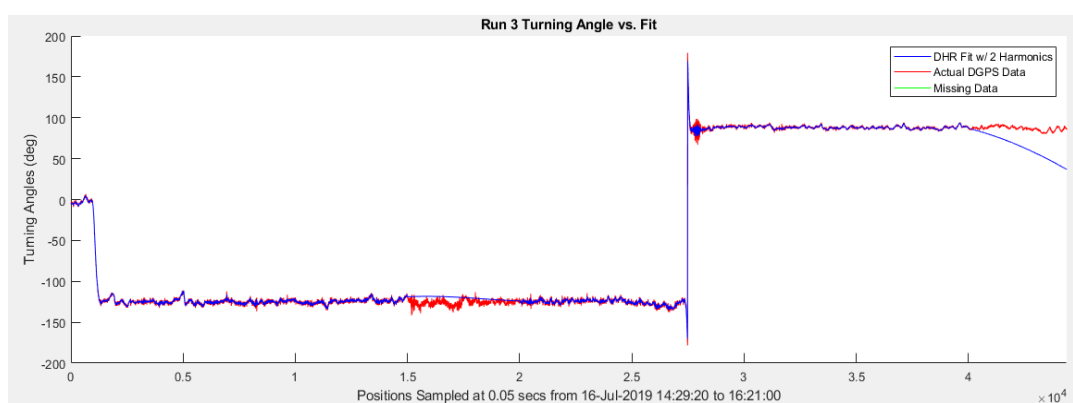
Fig. 55—DHR fit (blue) to actual Run 3 turning angle data (red). Missing data sections where the DHR interpolated and forecasted data lie between samples 15000 through 20000 and 40000 through 45100.
