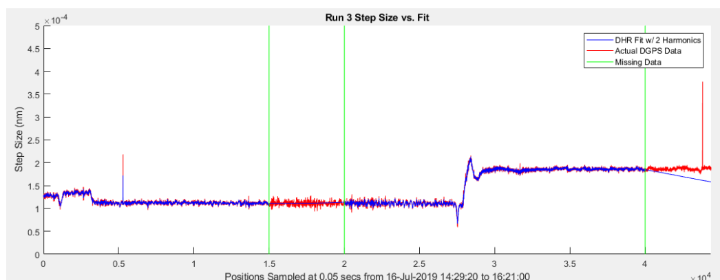
Fig. 53—DHR fit (blue) to actual Run 3 step size data (red). Missing data sections where the DHR interpolated and forecasted data lie between samples 15000 through 20000 and 40000 through 45100.
