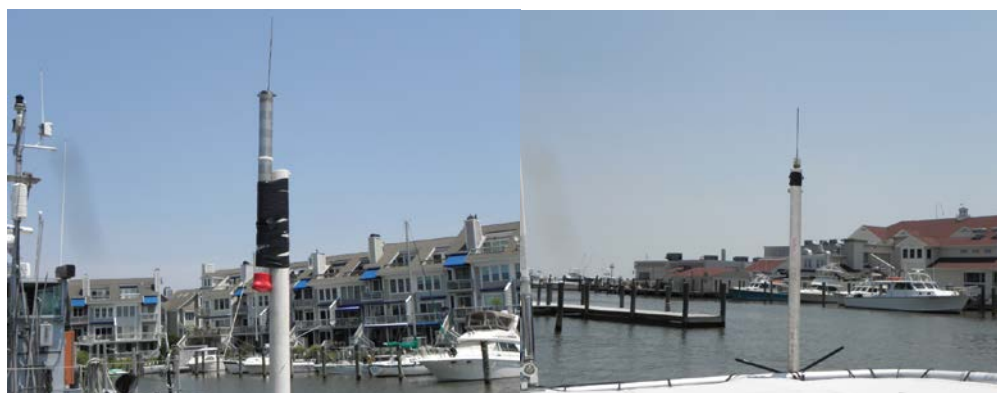
Fig. 24—SPOT 303C (left) and SPOT 258F (right) securely attached to vessel center console
