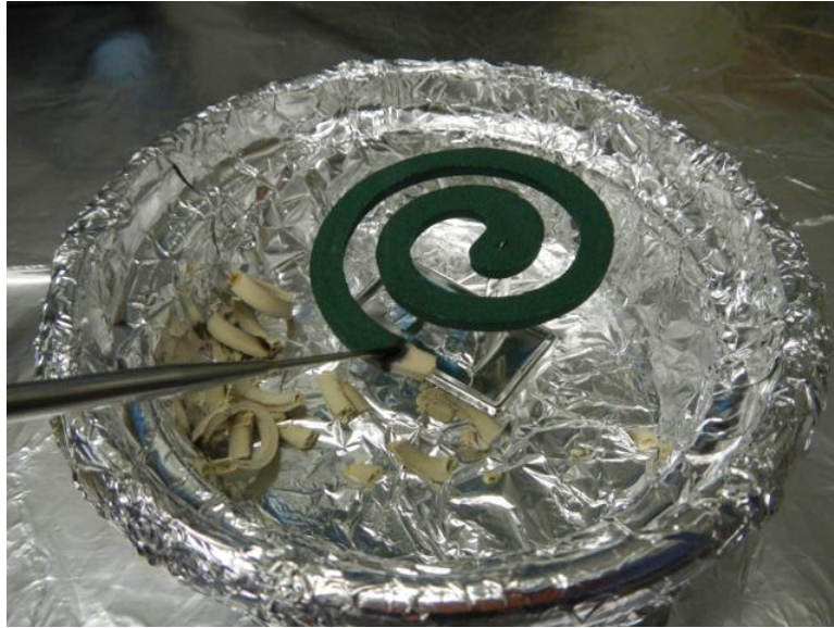
Figure 5. Illustration of the smoldering mosquito coil highlighting the region where the coil combustion temperature was measured
