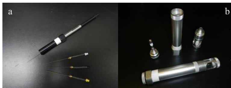
Figure 7. (a) SPME fibers and holder, and (b) SPME fiber storage container
