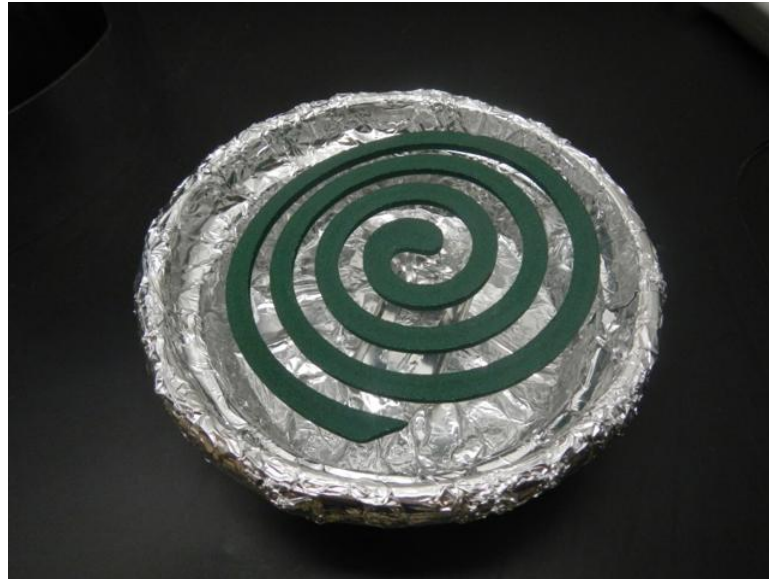
Figure 4. Sample mosquito coil in aluminum foil lined ash collection bowl
