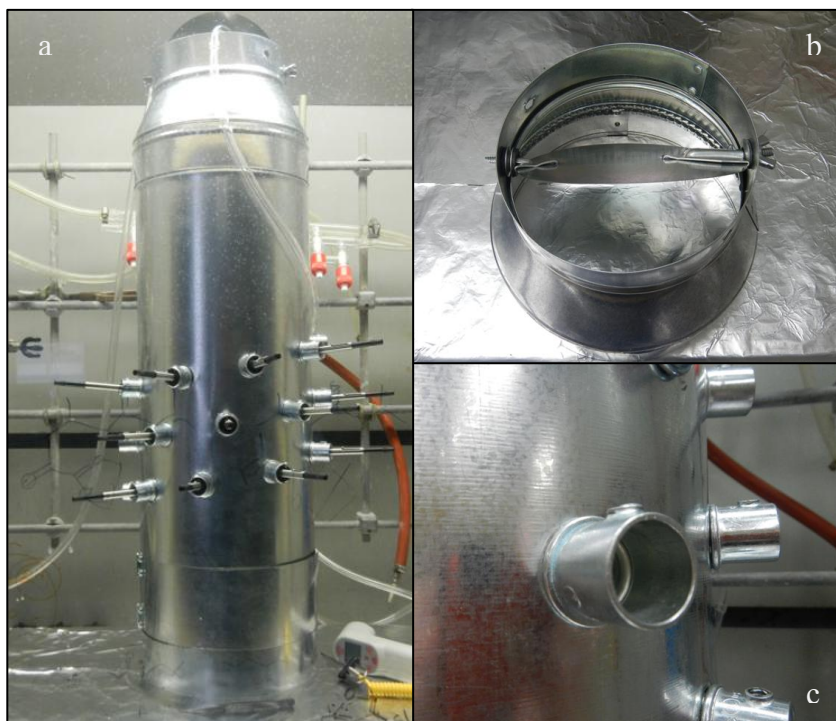
Figure 3. (a) “Smokestack” combustion chamber, (b) damper, and (c) sampling ports
