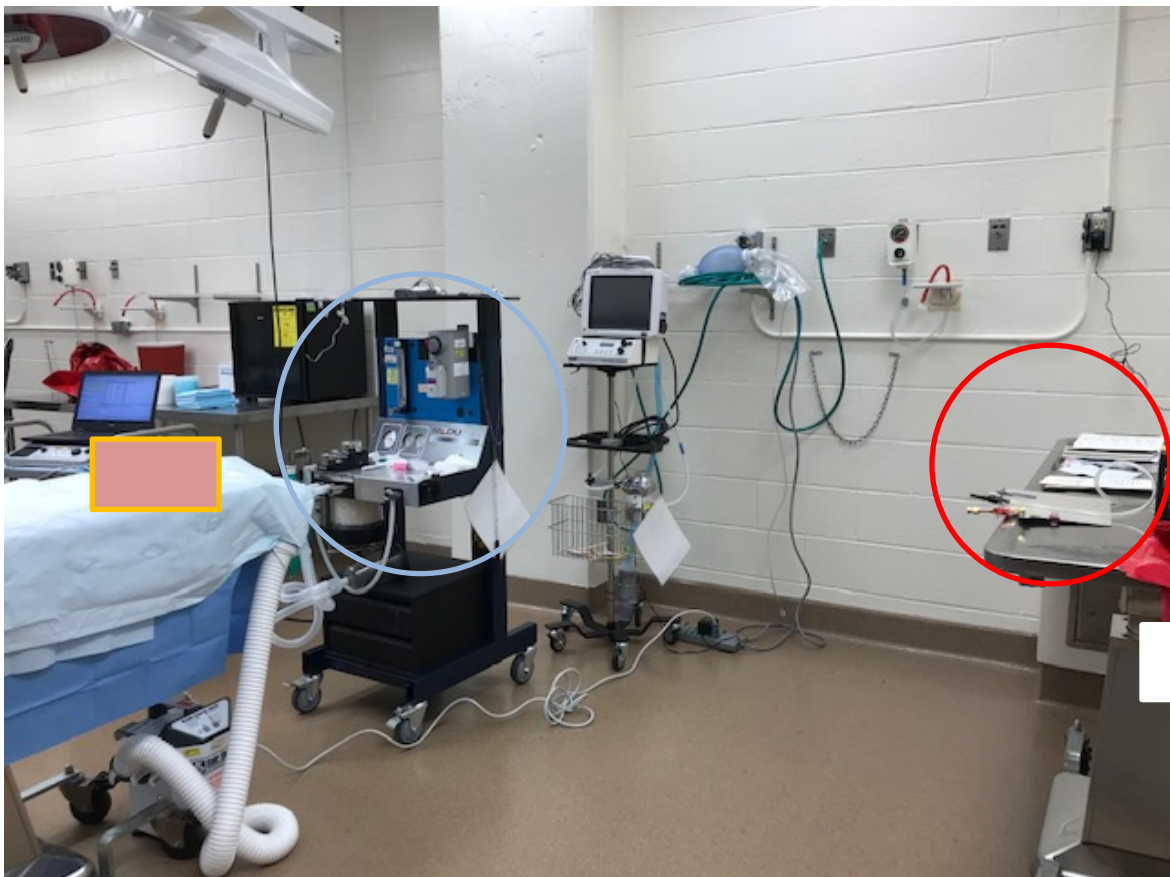
Figure 3.1. Common surgery area configuration for sampling. The blue circle shows the vaporizer and passive scavenging system, the red circle shows the location of the sampler set and the orange block shows the nose-cone/intubation area.
