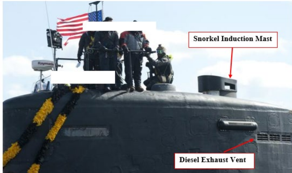
Figure 2: Sail configuration of a LA Class Submarine (17)
