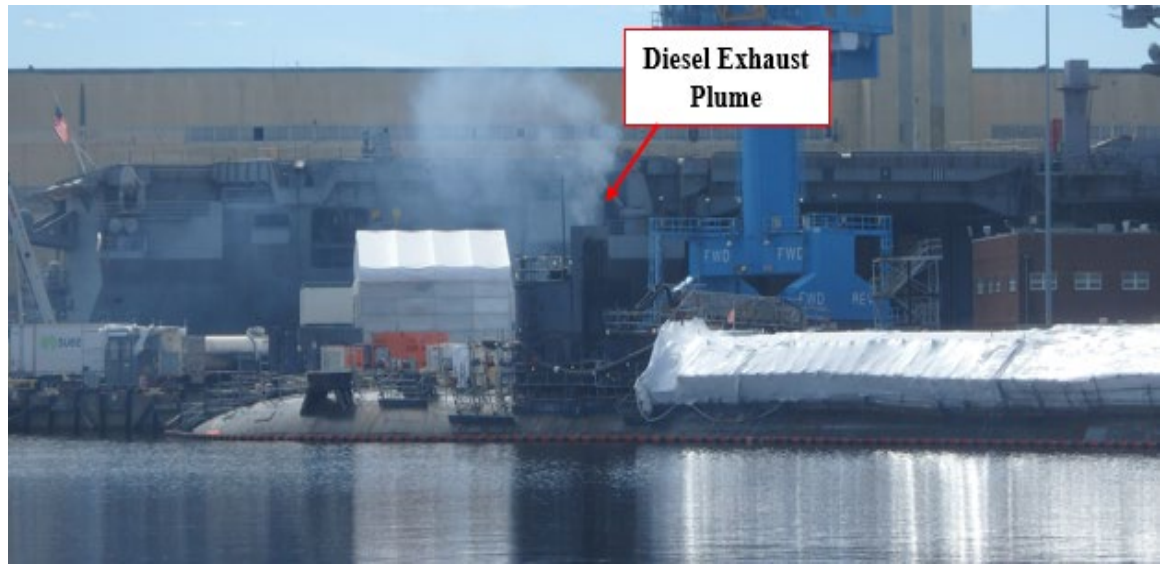
Figure 14: Submarine 2 Exhaust Plume from Modified Sail
