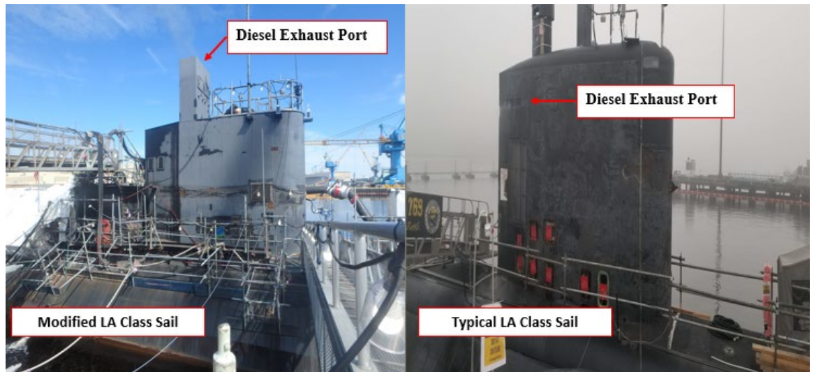
Figure 13: Submarine 2 Modified Sail vs. Submarine 1 Normal Sail
