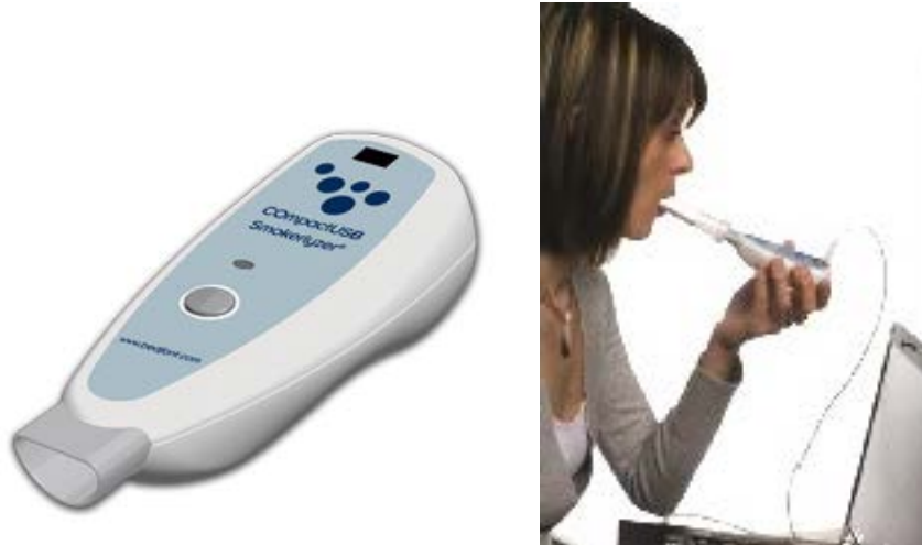
Figure 11. COmpact™USB device on the left and demonstration of its use on the right.
