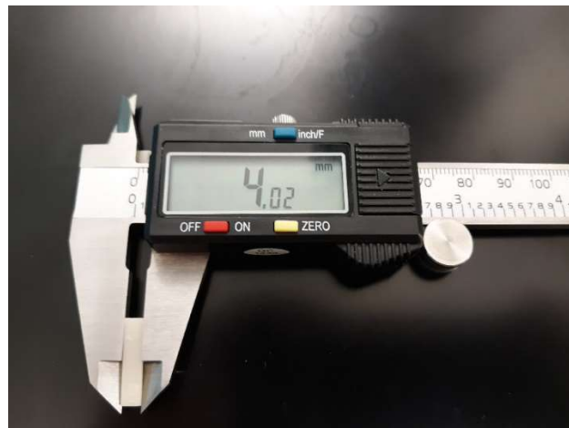
Figure 3. Measurement of STML bars
