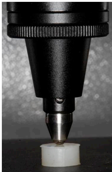
Figure 3: Samples were subjected to a load of 100 grams for 15 seconds by the Knoop hardness indenter.
