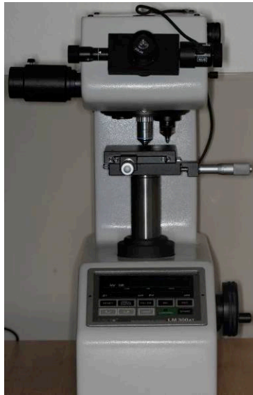
Figure 2: Surface hardness measurements were taken utilizing the Knoop hardness tester.
