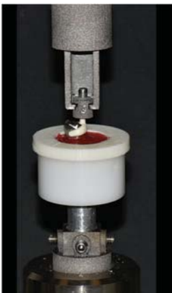
Fig. 6 – Mechanical load testing of clasp assembly.
