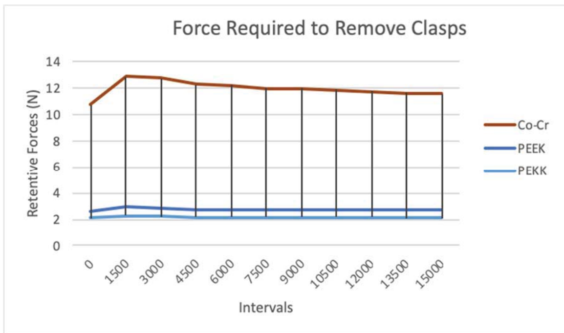
Fig. 7 – Mean force required to remove all clasps over 15,000 insertion and removal cycles.
