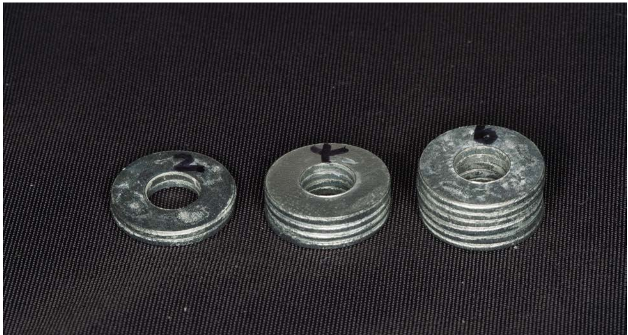
Figure 6. Spacers used to keep constant distance from the samples to the light tip
