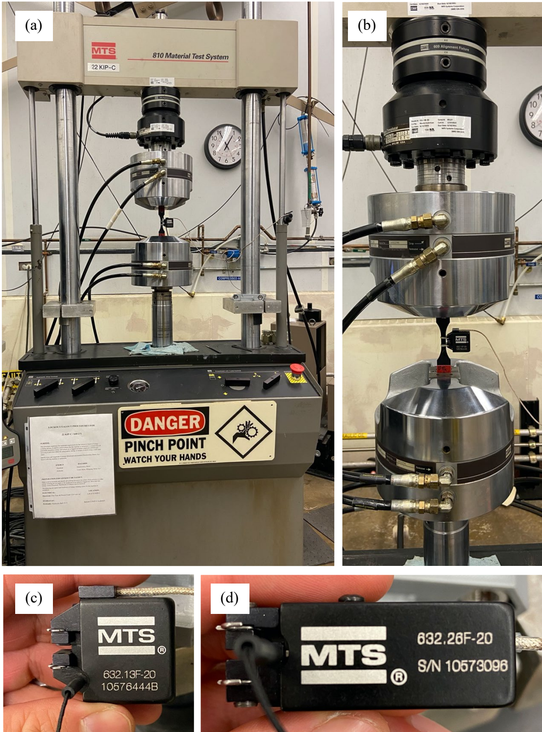
Figure 9: Picture of the: (a) MTS testing unit used to test samples, (b) load cell with sample, (c) 10-mm gauge Extensometer, (d) 8-mm gauge Extensometer.
