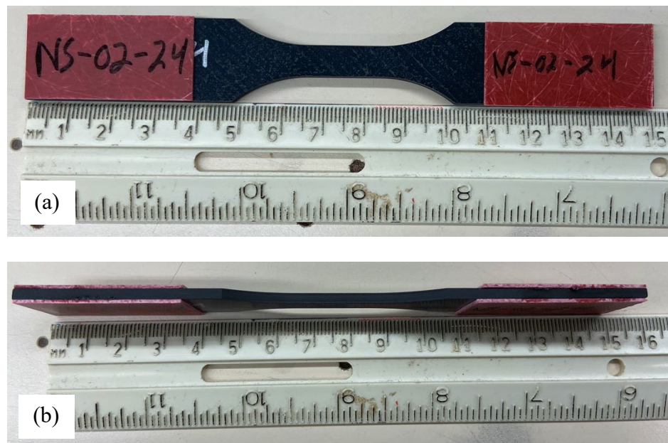
Figure 8: (a) Top and (b) side view of specimen with fiberglass tabs applied
