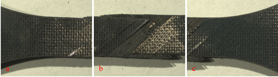
Figure 61: Images of the \pm 45 baseline composite specimen B-05-19 tested in tension to failure. (a-c) face view.
