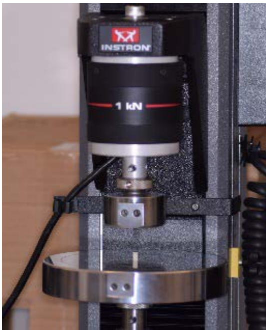
Image 3. Compressive Stress Test
