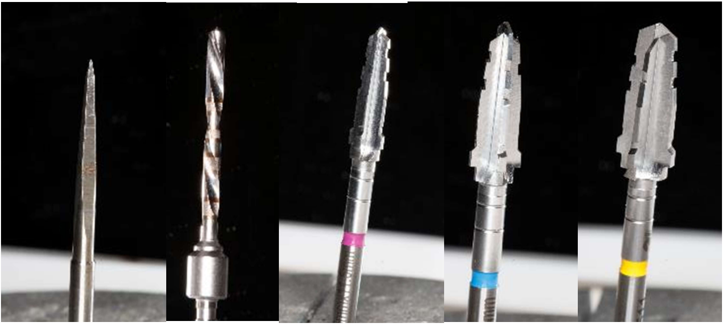
Figure 1: 3i Implant Osteotomy Burs (from left to right): pilot, 2mm twist, 3.25mm quad shaping, 4.1mm quad shaping, 5.0mm quad shaping.
