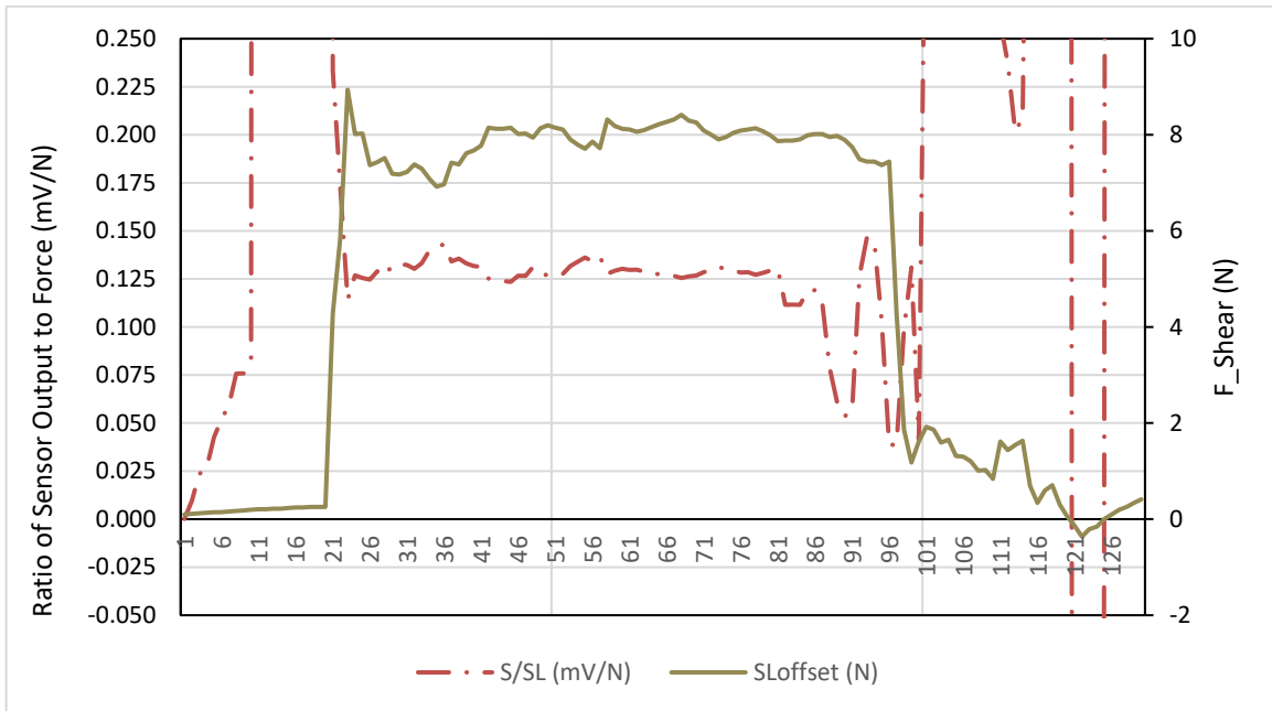
Figure 35: NSST-1 shear force calibration. S/SL is ratio of shear bridge output to applied shear load. SLOffset is applied shear force.
