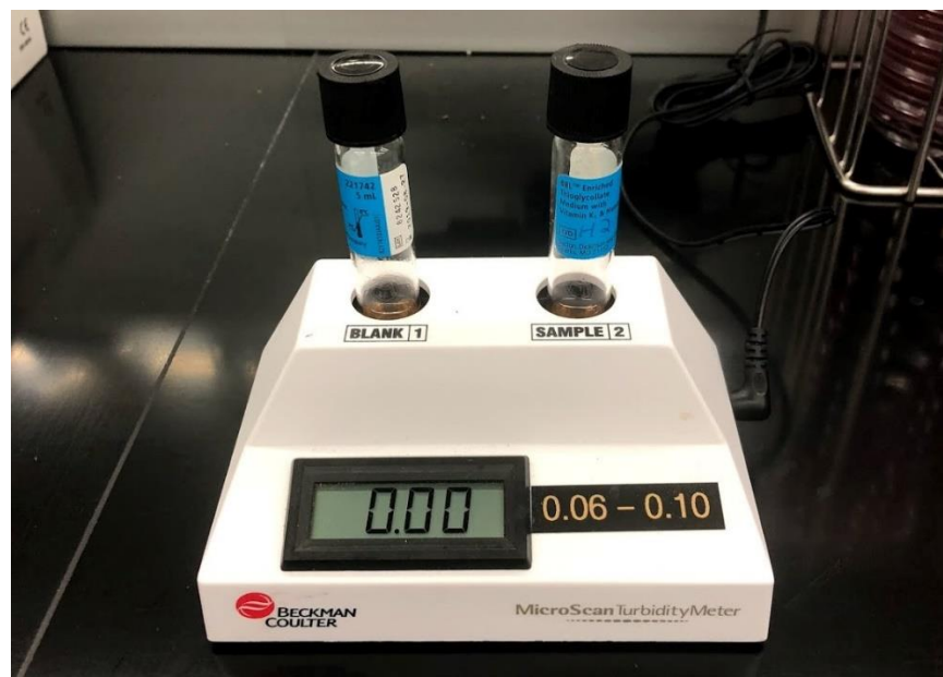
Figure 6 - MicroScan Turbidity Meter (Beckman Coulter Inc., Atlanta, GA) for recording OD readings, seen here is a DHS sample in a thioglycolate broth vile (right) calibrated against a new unused vile (left).
