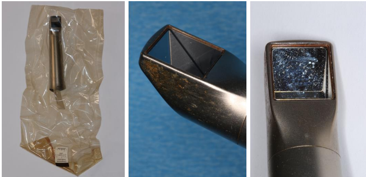
Figure 3 – Left, Omnicam mirror sleeve in sterilization pouch after DHS. Center and Right, Unwanted effects after long term dry heat cycling of the mirror sleeves, to include bioburden on sleeve and sapphire-coated glass.
