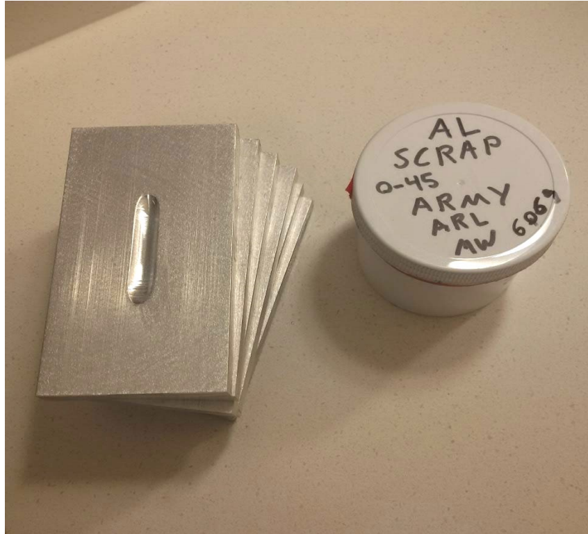
Fig. 22 AA6061 Al panels with simulated damage, and the Al powder (-325 mesh) made in the MolyWorks Mobile Foundry using scrap Al as the feedstock
