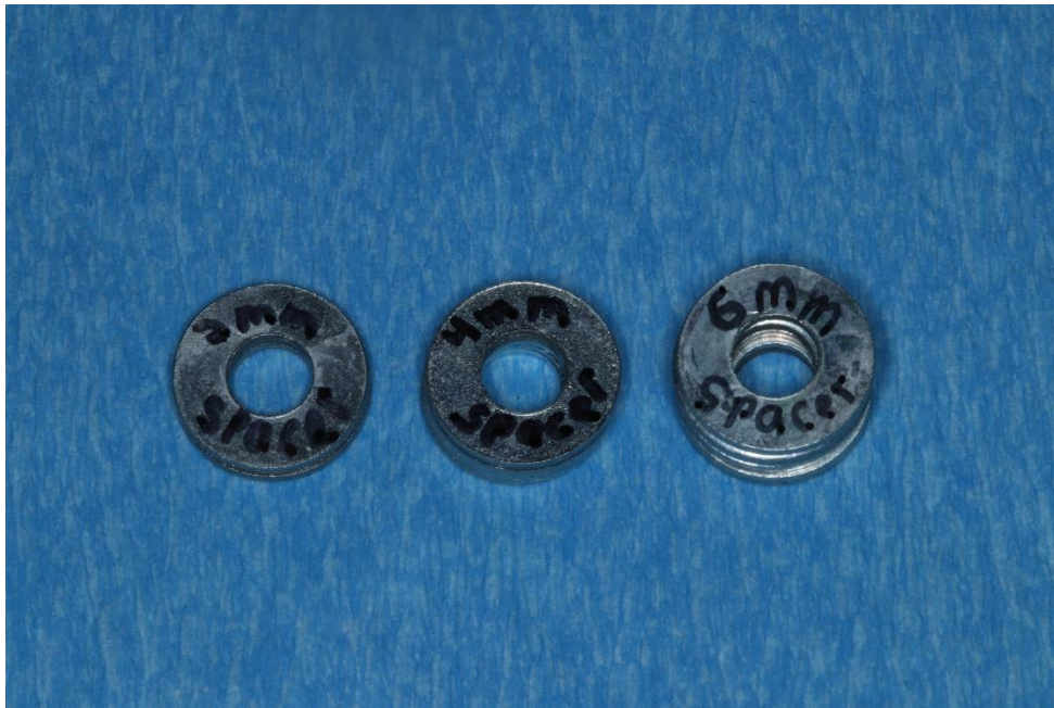
Figure 5: Spacers used to keep the curing light tip distance constant for each group. Starting from left to right, 2mm spacer, 4mm spacer, and 6mm spacer. The 0mm group did not require a spacer.
