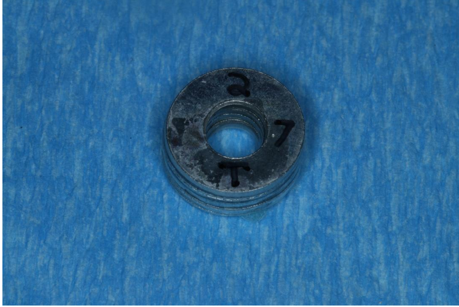
Figure 4: 5mm deep well consisting of 1mm stock washers glued together. The number 2 at the 12 o'clock position indicates a sample with a 2mm tip distance. The number 7 at the 3 o'clock position indicates it is the 7 th sample of the group. The letter T at the 6 o'clock position indicates the top side of the sample, which is closest to the curing light.
