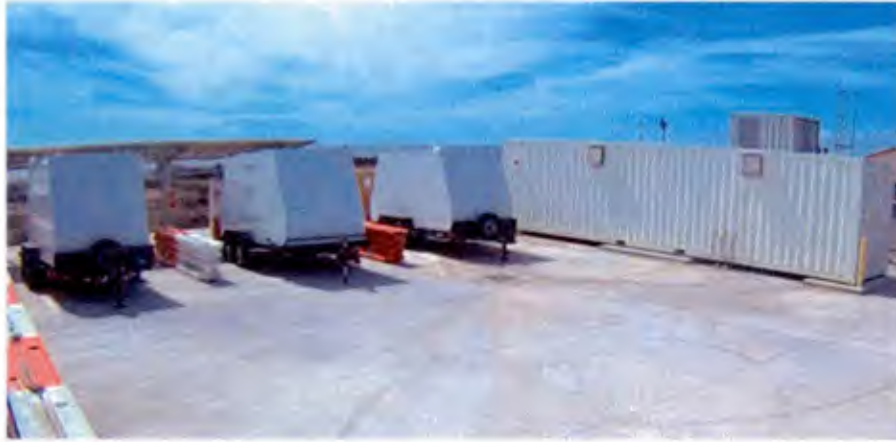
Figure 2.4.4. Hydrogen transport trailers.
