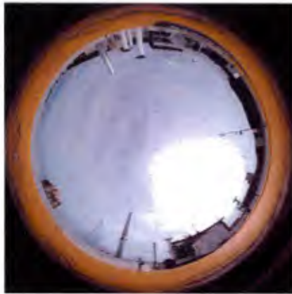
Figure 5.10.5. HNEI has developed new methodology for identifying and characterizing clouds in sky images. The method is able to better resolve cloud containing pixels near to the solar disk, while removing solar effects.
