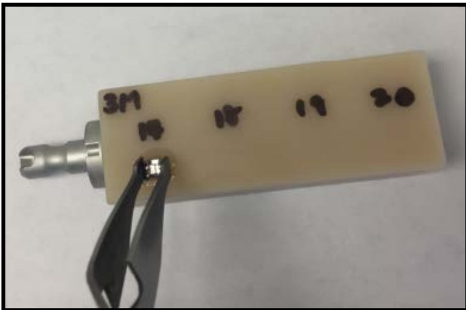
Figure 10: Transbond XT Light Cure Adhesive Primer Applied to PMMA Surface and Transbond XT Light Cure Adhesive Paste Applied to Bracket Base
