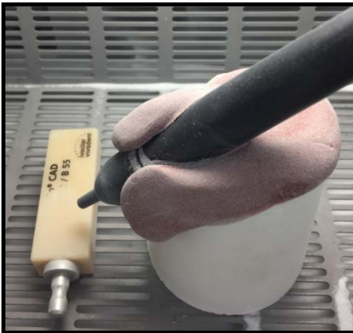
Figure 35: Abrasion Jig in Use
