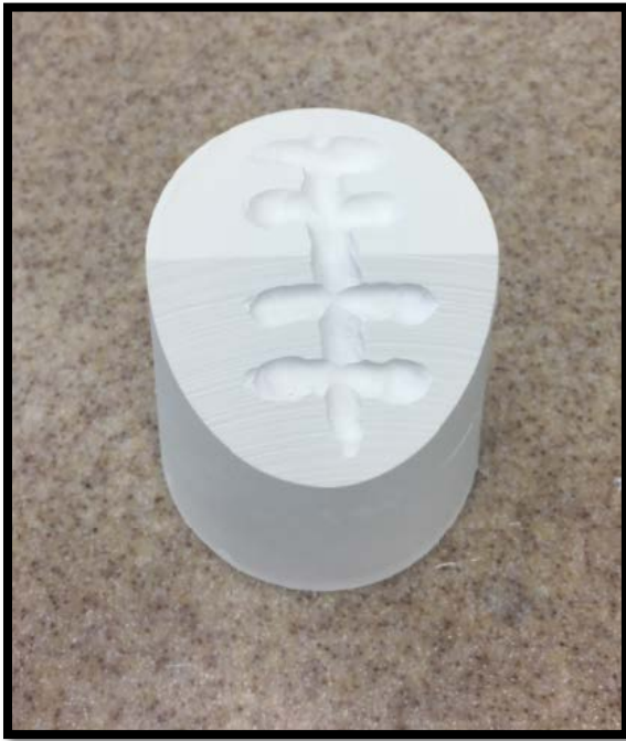
Figure 32: Retentive Grooves Cut
