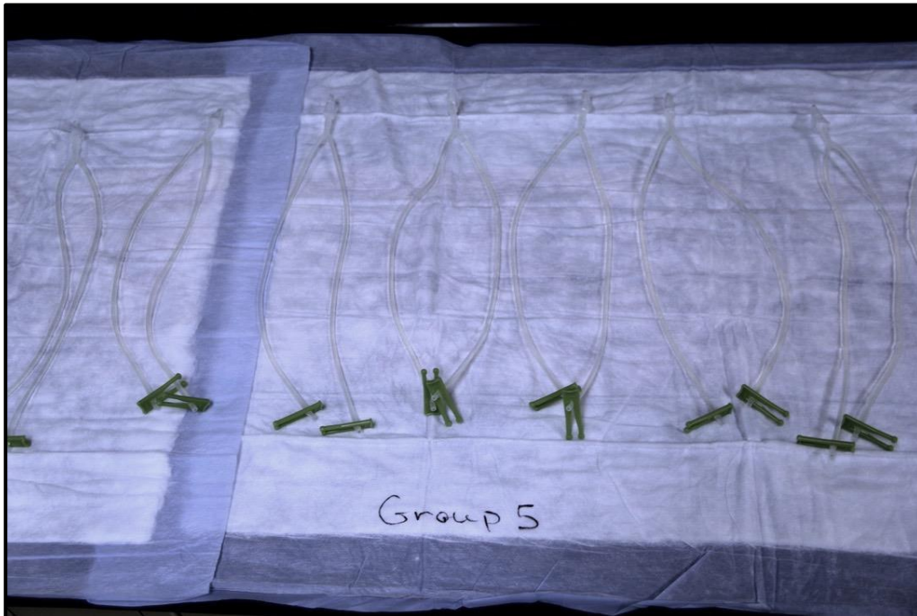
Figure 6. NOLA tubing samples on sterile drapes following inoculation during 2-hour delay period prior to processing for sterilization.
