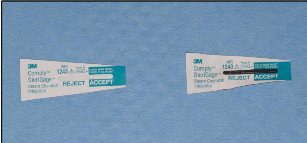
Figure 3. 3M Comply SteriGage class 5 biological indicator strips; unprocessed (left) and post-autoclave processing indicating successful sterilization (right).
