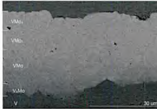
Figure 37: SEM image of Mo slurry coating using HPC on a V substrate.
