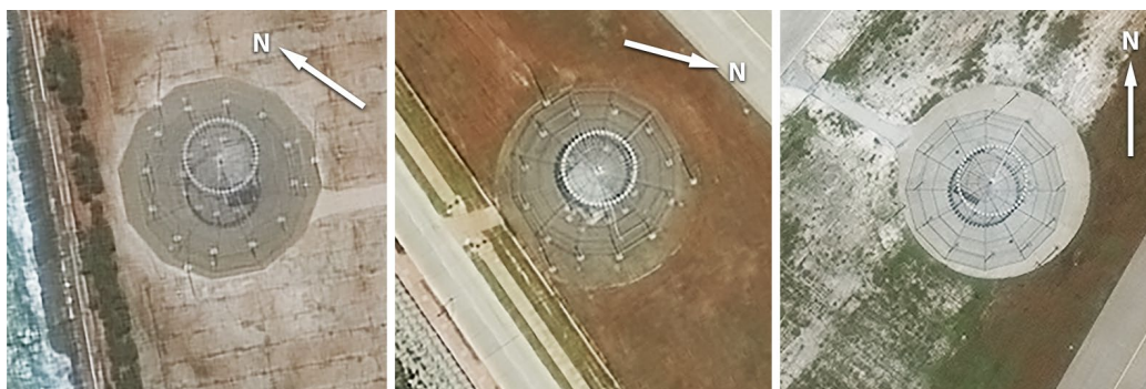
Figure 12. DVOR Sites Adjacent to Runways on Fiery Cross (Left), Subi (Center), and Mischief Reefs (Right)
