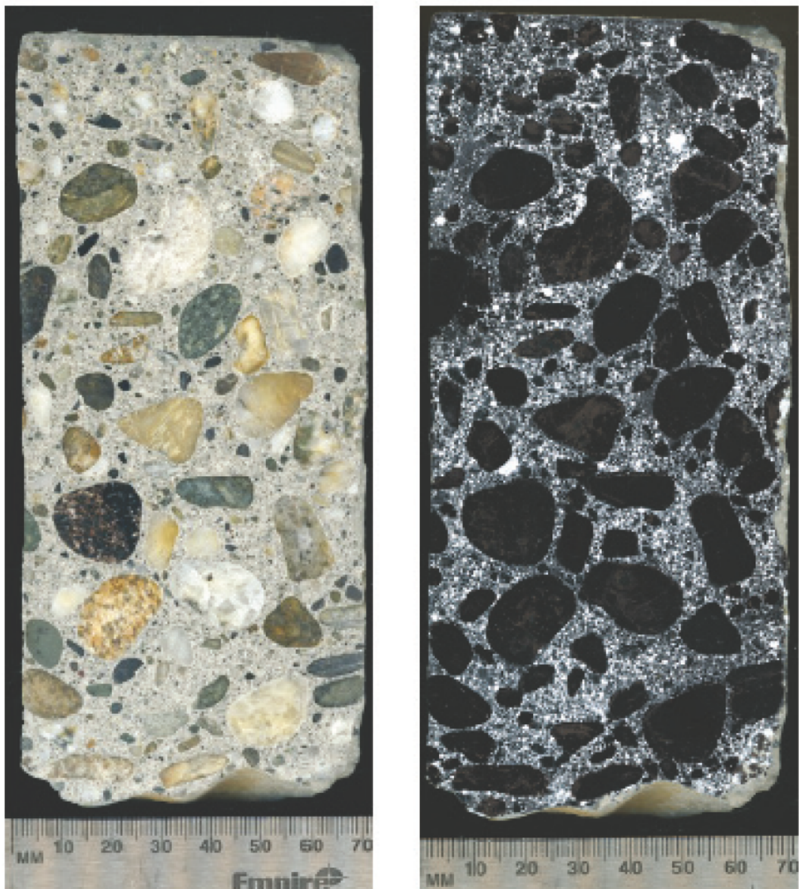
Figure C-12. Sample 12, hardened air-void analysis (23.05%).
