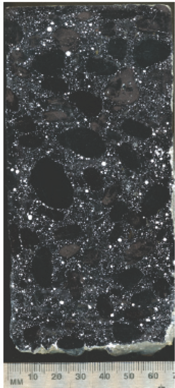
Figure C-11. Sample 11, hardened air-void analysis (9.57%).
