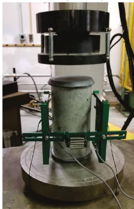
Figure 5. Modulus of elasticity test setup with extensometer.
