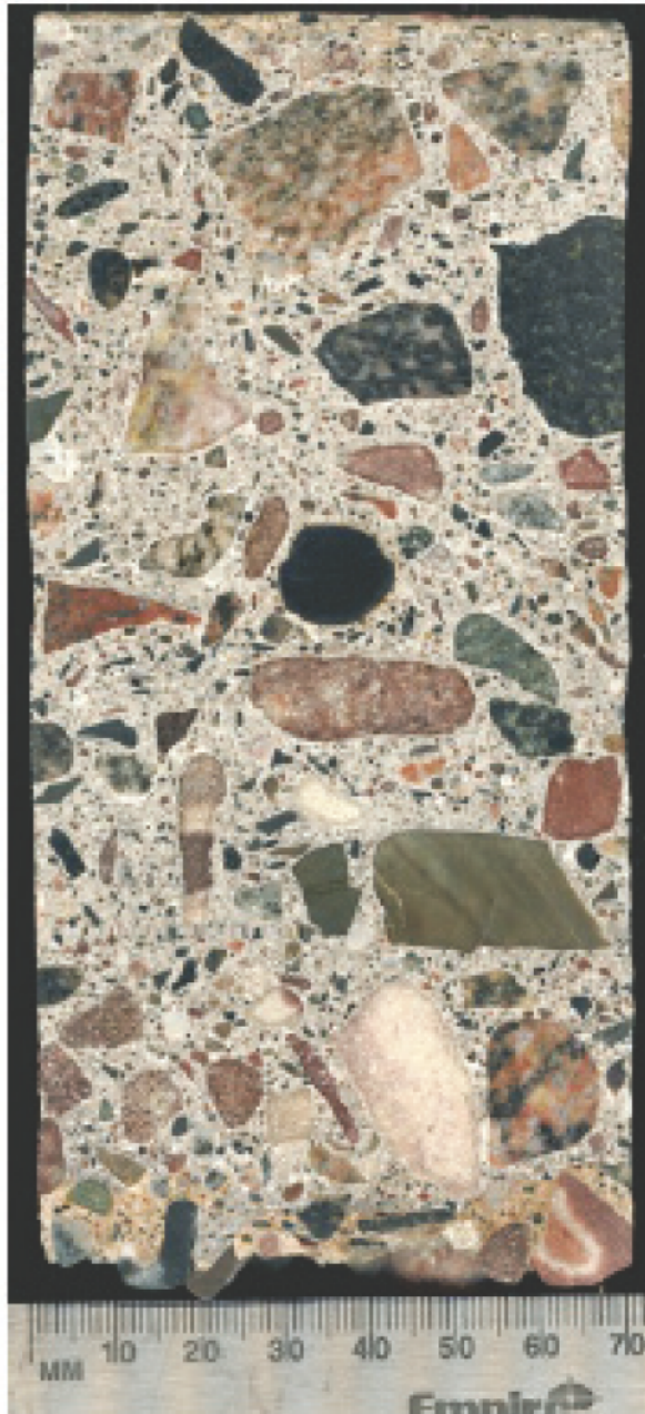
Figure C-1. Sample 1, hardened air-void analysis (4.59%).
