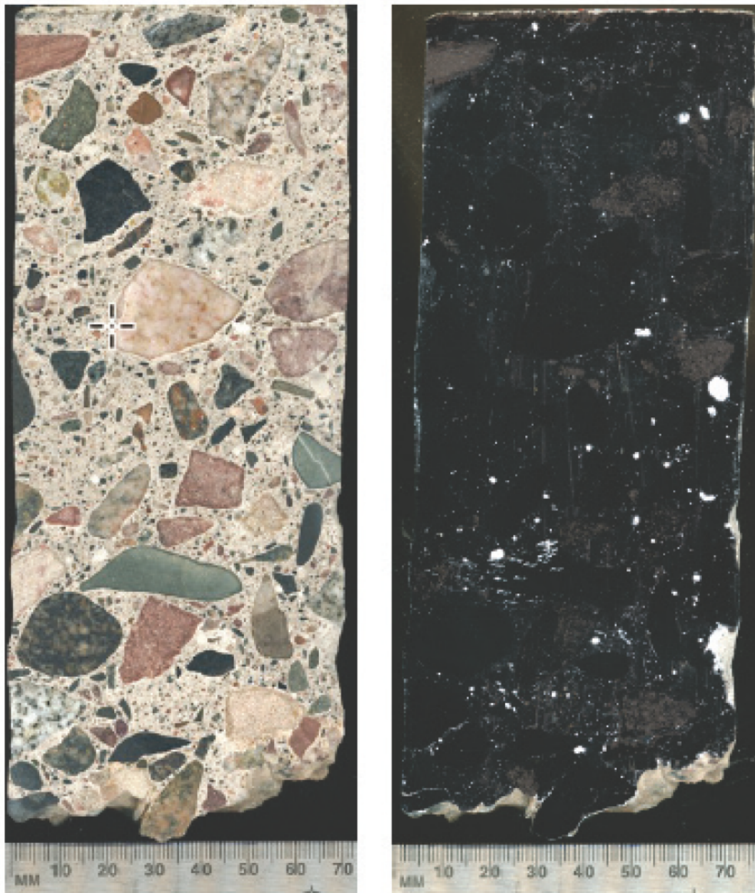
Figure C-2. Sample 2, hardened air-void analysis (3.87%).
