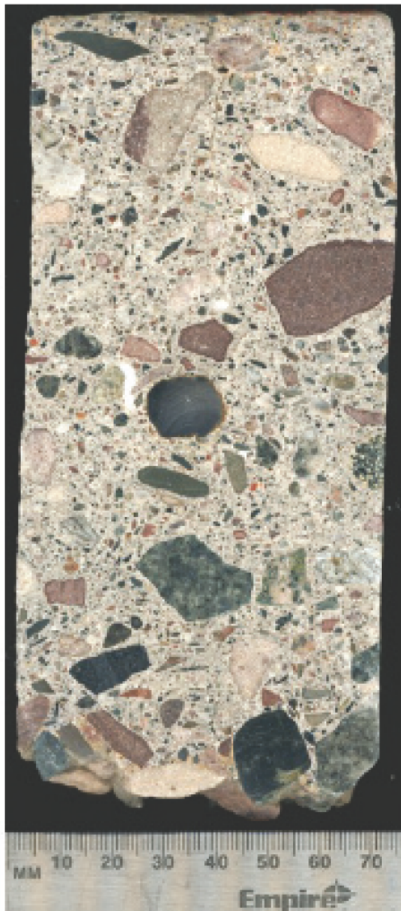
Figure C-3. Sample 3, hardened air-void analysis (9.47%).
