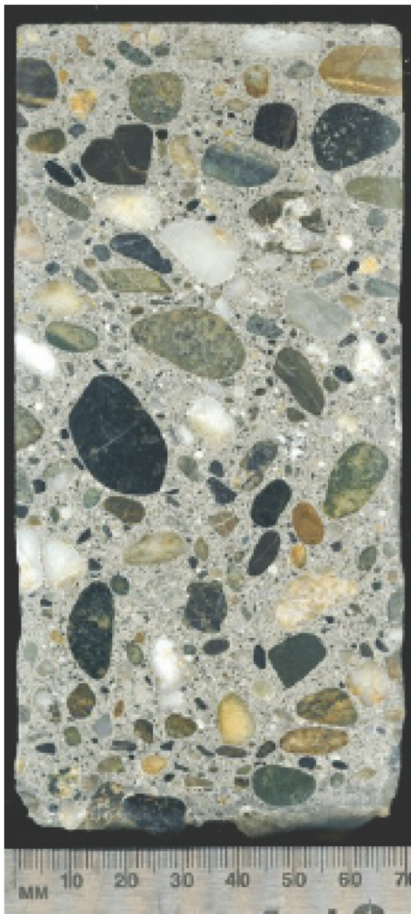
Figure C-11. Sample 11, hardened air-void analysis (9.57%).
