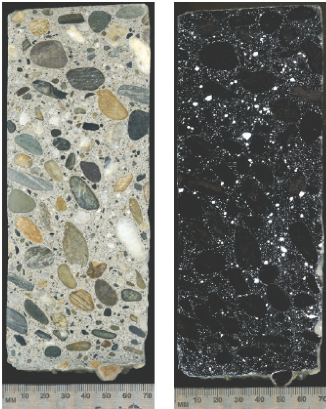
Figure C-10. Sample 10, Hardened air-void analysis (9.24%).
